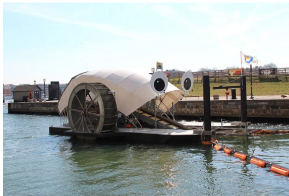
Image 2: Water powered machines like Mr Trash Wheel, use solar power provided from solar panels on his back to power a water wheel to help him pick up trash.
