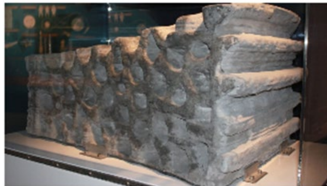
Fig. 4 - A 1.5 tonne building block of artificial lunar regolith, demonstrating 3D printing using lunar soil 15
