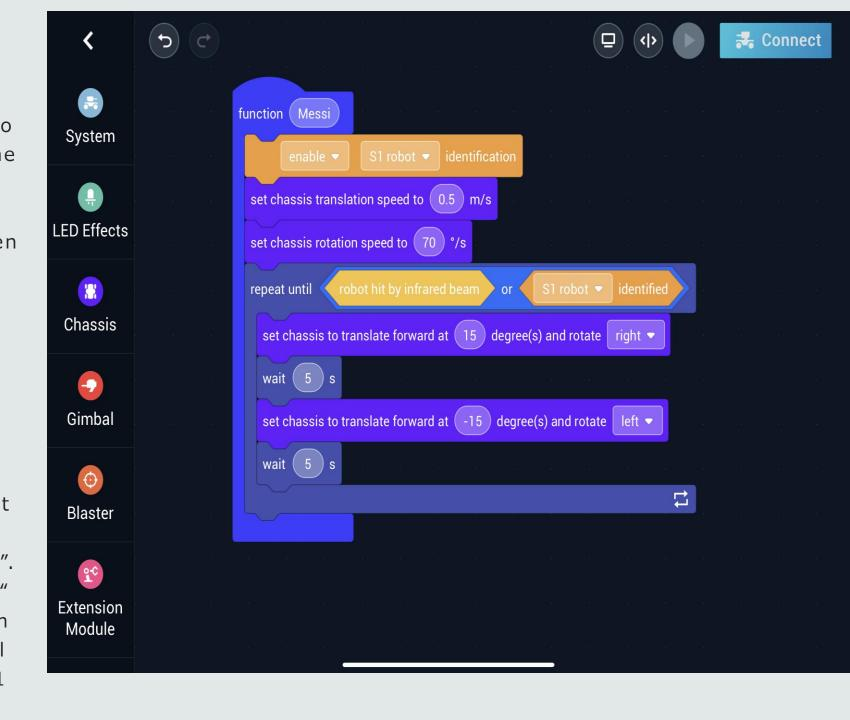
In this part this what happens when the program starts, first it is "enable s1 robot identification" so the program allows the robot to identify the other robot. Then the program does the function "messi" (slide 17) the "messi" will be put in an always so the program won't stop.
