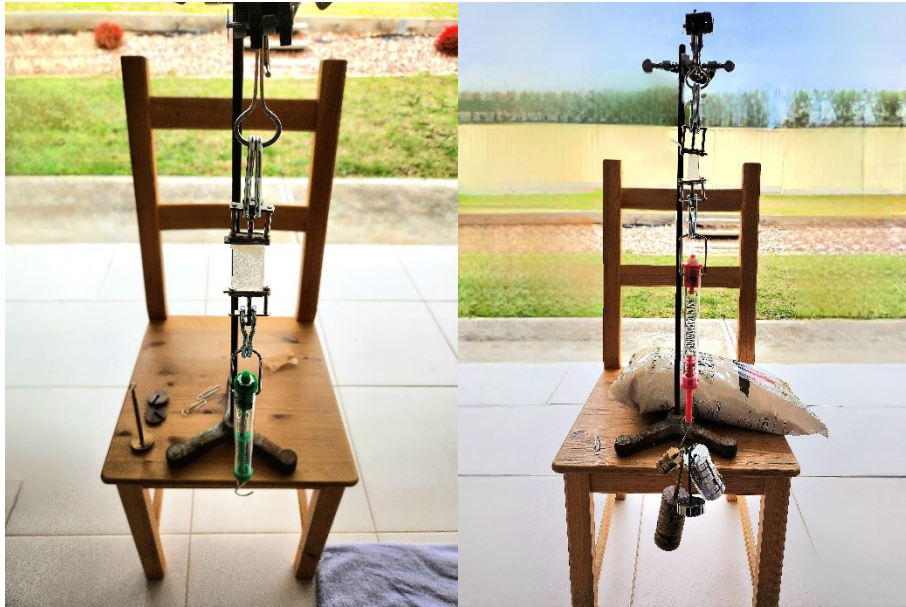
Figure. Tensile testing setup for samples A and B.
