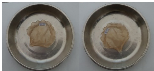
Figure d. Both recipes G and M shrinking to 1/3 size with no mold growth after 3 days of drying and heating.
