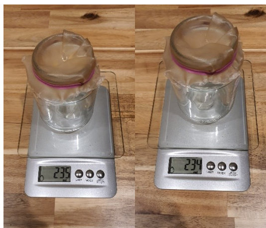
Figure. Water permeability test – pilot study B before and after 1 hour.
