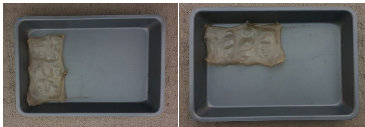
Figure a. Recipe G shrinking to 1/3 size after 3 days of drying and heating.
