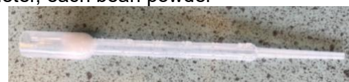
Figure 6: Cotton pipette filter used to remove undissolved bean powder particles from suspension
