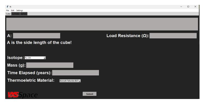
This is a later version of the GUI, whilst the design stayed similar, there were many differences. First of all, the pyramid tab was removed and the VXS Space Logo was added. The main part of the update was the new inputs which supported a more accurate output and allowed potential for power output calculation.
