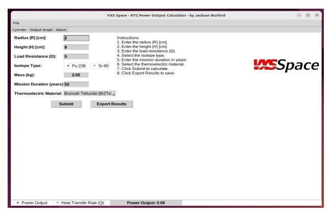
This is what the application looks like filled in (The Mass input has been removed since the screenshots have been taken because the Mass is calculated by Radius, Height and material.) The power output can be viewed in the grey box at the bottom.
