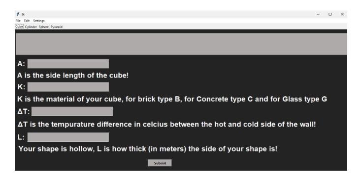
This is the first version of the GUI, works the same as the previous version except the temperature difference is now in celsius. The output would not work in this version.
