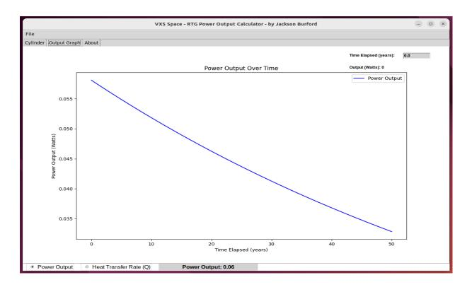
This is the output graph tab that shows the power output over time. You can see that the Y-Axis is the Power Output in watts while the X-Axis is the Time-Elapsed in years.
