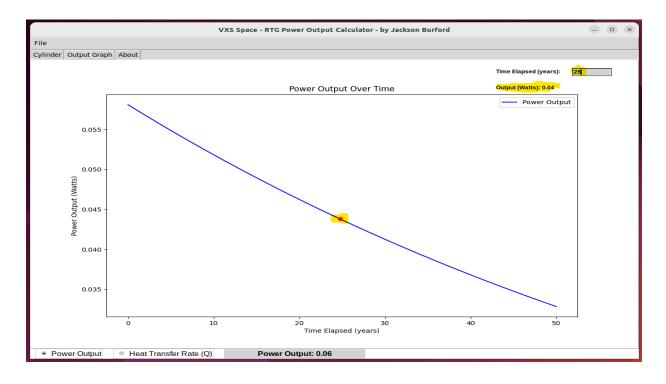
Here is the graph with the time elapsed option, you input how far you are in the mission and it shows the power output at that time and where on the graph you are.
