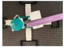
Then, in a forever loop, it sets the motor speed to the slider position, and then starts turning the motor. It also shows the slider postion on the circular dial. It shows angular velocity Z, which the hub measures, on the display labeled Z. After that, it does this velocity calculation, and shows the answer on the display labeled V:
