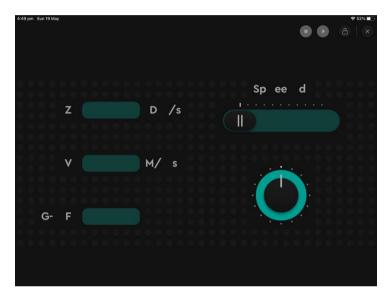
To use the centrifuge, you first move the slider, marked 'speed' to spin the centrifuge at the speed you want. The circular dial will show the speed. If you look at the display marked 'g-f' it will show the amount of g-force that is being put on the astronaut figure. The display marked 'V' shows the velocity, which is metres per second, of the spinning part. The display marked 'Z' shows angular velocity Z, which is degrees per second.
