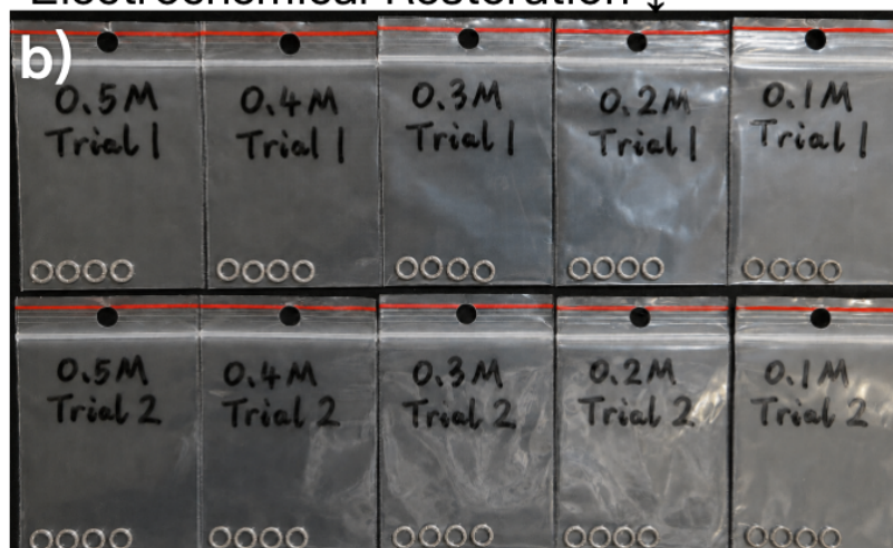
Figure 7. Comparison of tarnished and restored sterling silver samples. (a) Samples after sulfur tarnishing. (b) Samples after electrochemical restoration.
