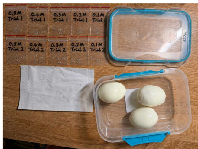
Figure 1. Pre-experimental setup for inducing tarnishing on sterling silver samples. Labeled samples are organized by concentration and trial, ready to be exposed to sulfur vapor from hard-boiled eggs.
