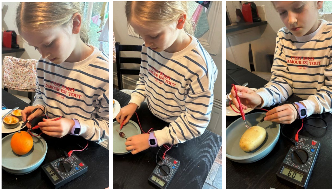
Figure 3 – Testing voltage produced by an orange, grape and potato
