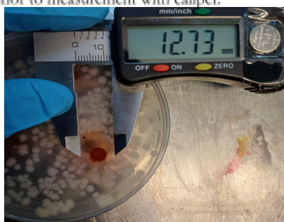
Fig. 13. Measurement of observable ZoI across two axes using digital caliper ( \pm 0.01\text{mm} uncertainty)
