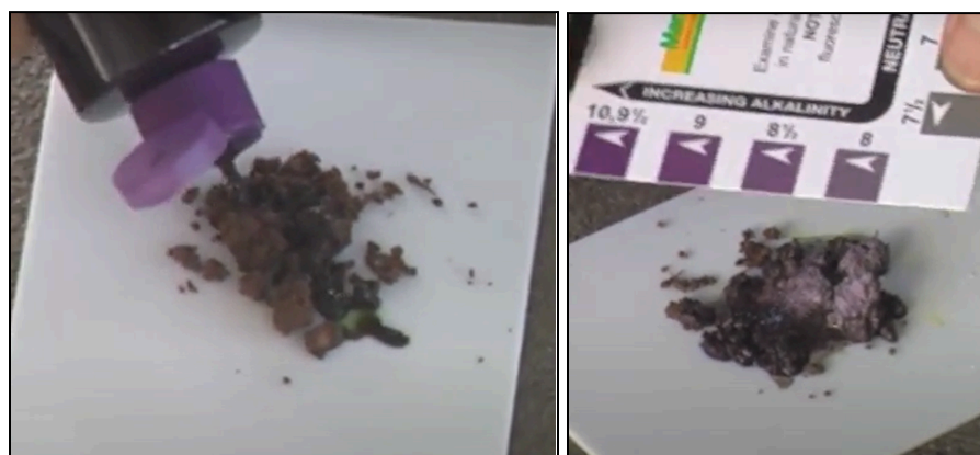
Figure 8: Soil mixed with indicator (left) & Color change comparison (right) - Manutec Youtube channel
